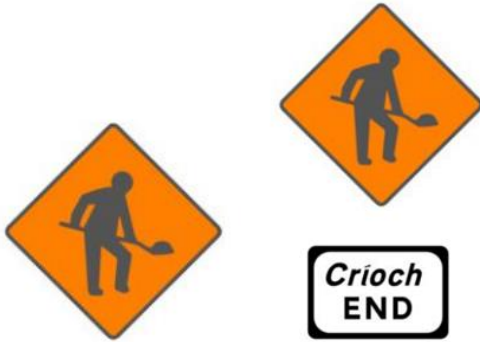
WK 001 - Roadworks Ahead / End
